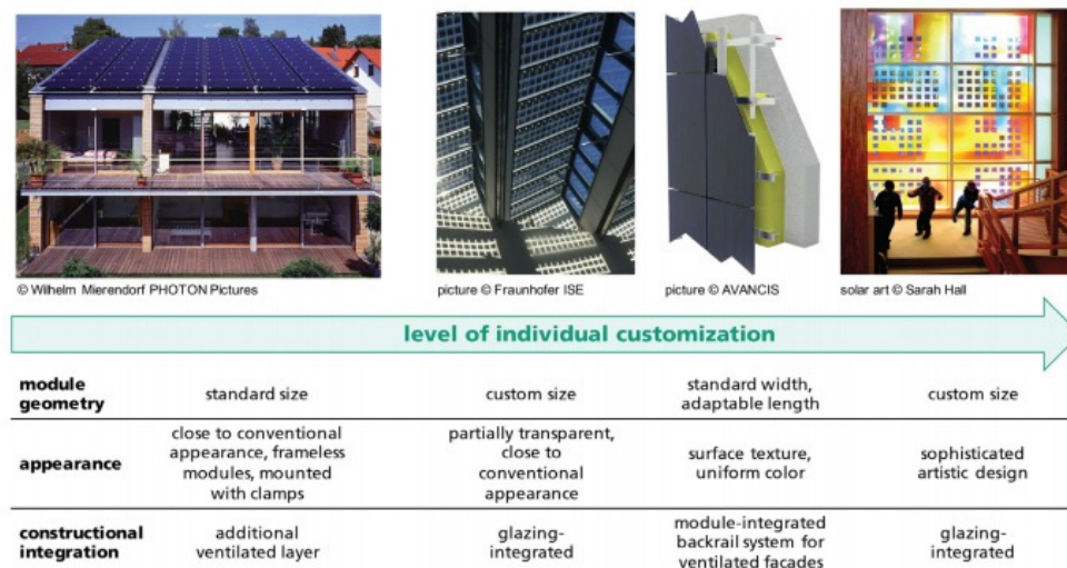
Figure 1: Overview of BIPV systems through examples [2]
