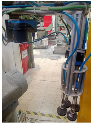
Figure 7: Proposed Zone-Based 2.5D Guidance System: Flat sideways camera, suction cups with movement compensation, new scanning method
