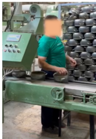
Figure 2: Worker manually depalletizing pots
