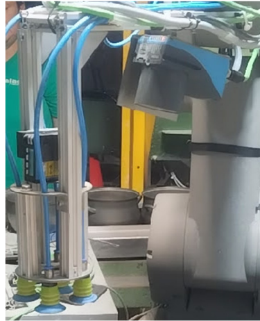
Figure 5: Improved EOAT Design: Quadruple-Vacuum + laser distance sensor + Angled Camera
