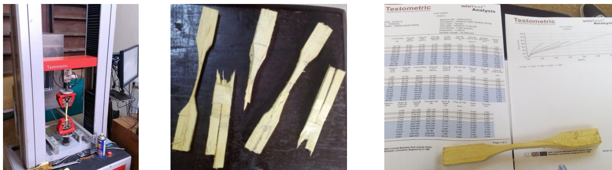
Figure 6: Universal testing machine under tensile test and data
