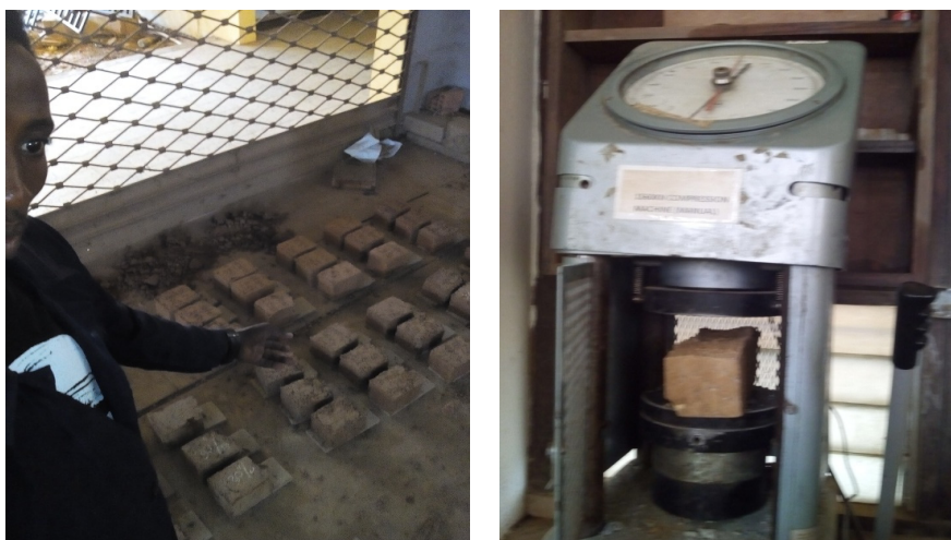
Figure 3: Compressive testing machine
