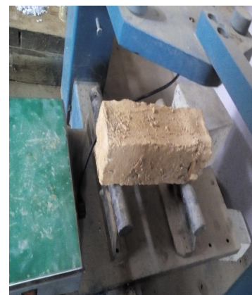
Figure 9: Modulus rupture test and ruptured samples
